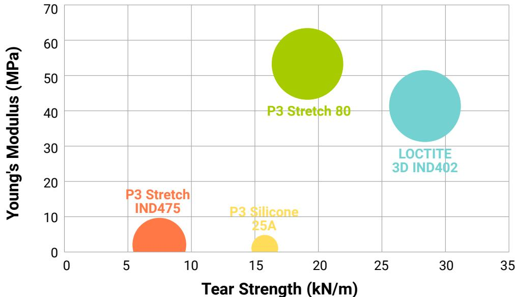
Higher Young's Modulus values indicate that the material is stiffer and has a higher Shore Hardness value. Elastomers with higher stiffness are generally more resistant to tearing.
