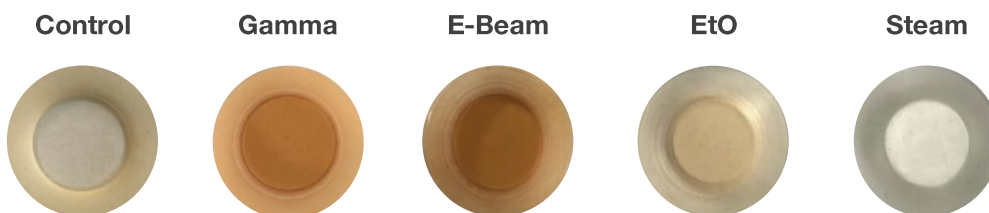
Color discs before and after sterilization
