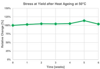
ASTM D638: Type IV, Pull speed: 5 mm/min, Young's modulus measured at 0.1-1.0% (regression),  $22^{\circ}$ C
