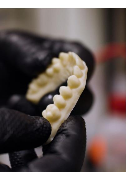
Origin One Dental's P3 technology utilizes computer vision and 25+ environmental sensors to monitor and respond to every aspect of the print process. In situ analytics, combined with automatic pressure, pull force and temperature regulation ensure the first part is the same as the last. See powerful product improvements over time, with over-the-air software updates that unlock new advanced materials and workflow optimizations.
